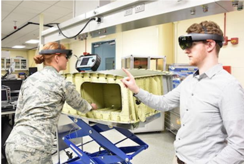
Fig. 7 AFRL researchers demonstrate augmented reality for aircraft inspections, presenting all essential information in the user's field of view, streamlining the process.
