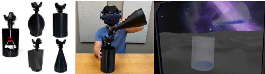
Fig. 12 Geppeteau employs a pulley system based on strings to dynamically adjust the center of gravity of a vessel, creating haptic feedback sensations of virtual fluids. This technology has the capability to enhance various common vessel profiles, as illustrated by four sample vessel shapes on the left. Users in any physical environment (middle) can engage with virtual fluids in simulated settings (right) [76]
